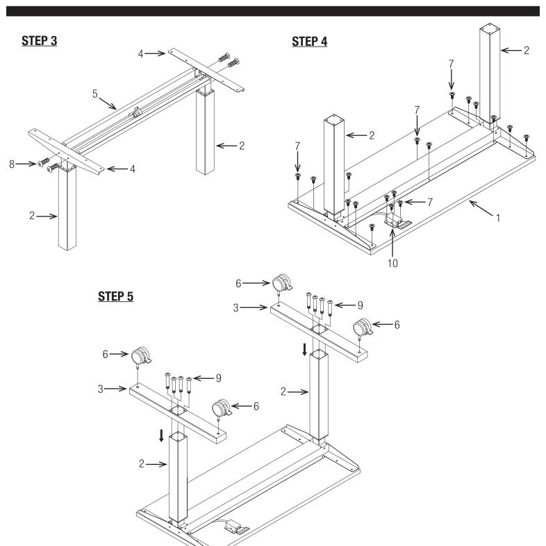
STEP 3 Attach Top Supports (4) to Leg Posts (2) using two Medium Bolts (8) for each Leg Post (2). FULLY ALL BOLTS USING ALLEN WRENCH (11).
